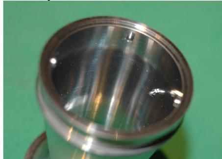
Insert the air-valve in the rear rim. Holding it in place, use water thin superglue applied to the back side where it protrudes through the rim and let it "wick" in.
